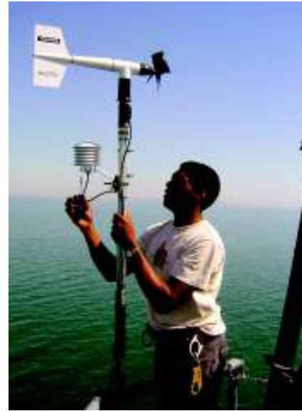
National Weather Service observation platform being installed at the lighthouse in Safinaw Bay, Michigan (Image credit: NOAA)
