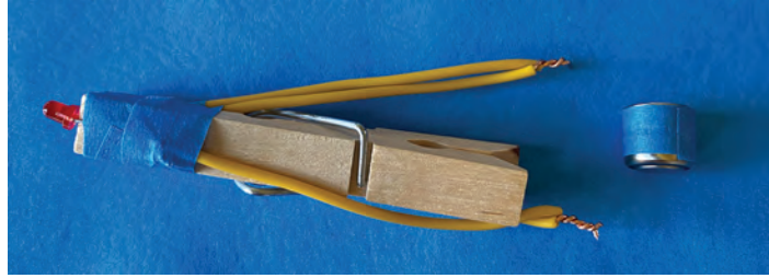
Figure 10: Positive and negative wires twisted together
